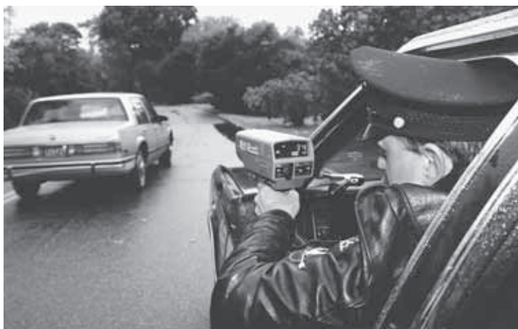
Police officers often use radar to detect the speed of a car. The radar gun is used to determine whether a car is traveling faster than the speed limit.
