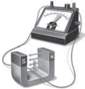
As the wire moves between the poles of the magnet, it cuts through magnetic field lines. This induces an electric current.
