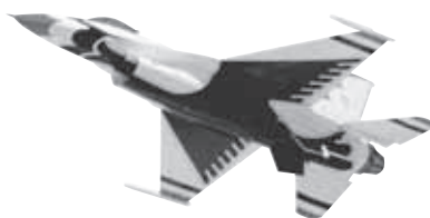
The engine of this jet creates a large amount of thrust, so the wings don’t have to be very big.
