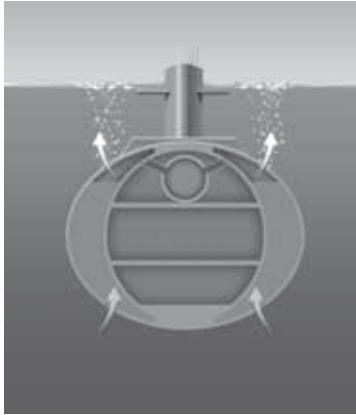
Water flows into the ballast tanks. The submarine becomes more dense and sinks.
