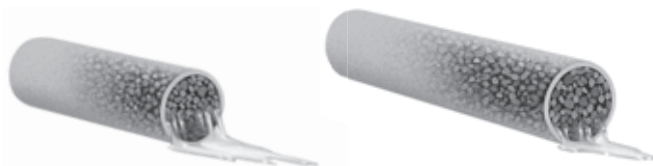
A short pipe has less resistance than a long pipe does. This is because the water in a short pipe does not have to move around as many pieces of gravel.
