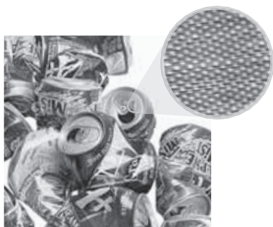
Aluminum cans are made of atoms. Aluminum atoms can be seen in the image from a scanning tunneling electron microscope (STM). Notice the regular, repeating pattern of the aluminum atoms.
