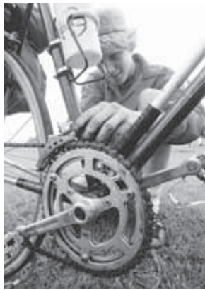
If you work on a bicycle, you may get dirty from the chain oil. This lubricant reduces friction between sections of the chain.
