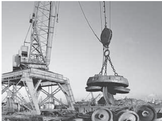
Electromagnets used in salvage yards are turned on to pick up iron objects and turned off to put them down.
