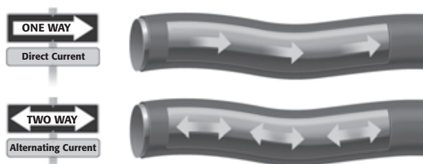
Charges move in one direction in DC, but charges continually change direction in AC.
