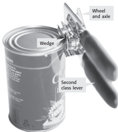
A can opener is a compound machine. The handle is a second-class lever, the knob is a wheel and axle, and a wedge is used to open the can.
