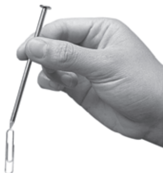
This nail was magnetized by dragging a magnet down it many times.
