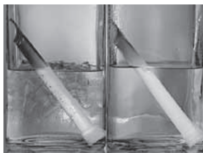
The light stick on the left is in cool water. The light stick on the right is in warm water. The higher temperature causes a faster reaction rate that produces more light.
