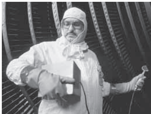
Tracers are used to find weak spots in materials and leaks in pipes. A Geiger counter is often used to detect the tracer.
