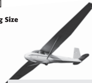
This glider has no engine and therefore no thrust. So, its wings must be large in order to maximize the amount of lift achieved.
