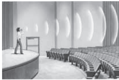
You would not hear an echo in this auditorium. The sound waves do not reflect as easily from the soft, uneven surfaces of the seats and walls.
