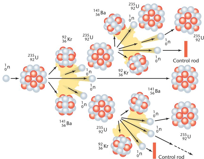
**FIGURE 31–5** The nuclear fission chain reaction of uranium-235 takes place in the core of a nuclear reactor.
