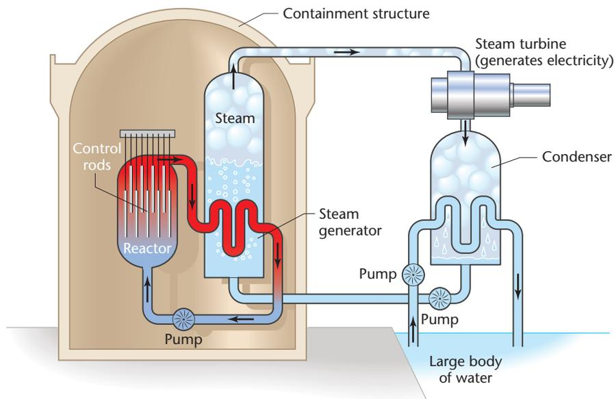
**FIGURE 31–6** In a nuclear power plant, the thermal energy released in nuclear reactions is converted to electric energy.
