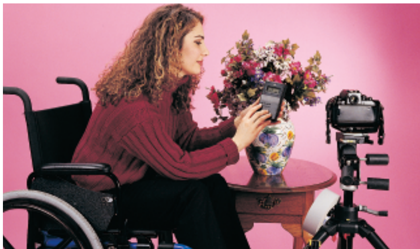
FIGURE 29–8 Photographers sometimes use a light meter to measure the intensity of incident light on an object. The meter converts the measurement into a unit that tells the photographer what exposure to set on the camera.
