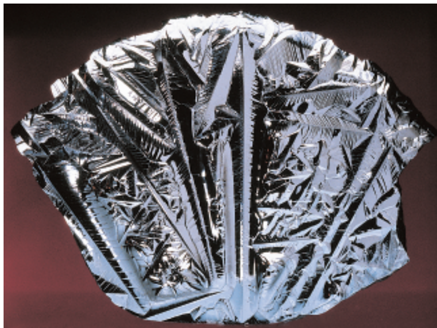
FIGURE 29–15 A piece of ultrapure silicon forms the basis for an integrated circuit chip.
