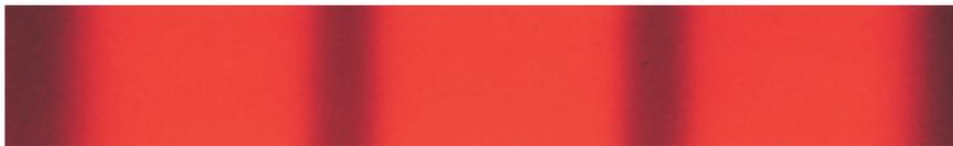
**FIGURE 19-5** This diffraction pattern for red light was produced with a single slit having a width of 0.02 cm.
