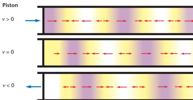
**FIGURE 15–1** A vibrating piston produces sound waves. The dark areas represent regions of higher pressure; the light areas represent regions of lower pressure. Note that these regions move forward in time.
