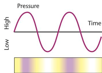
**FIGURE 15–2** A graphic representation of the change in pressure over time in a sound wave is shown. Dark areas indicate high pressure; yellow areas indicate average pressure; white areas indicate low pressure.
