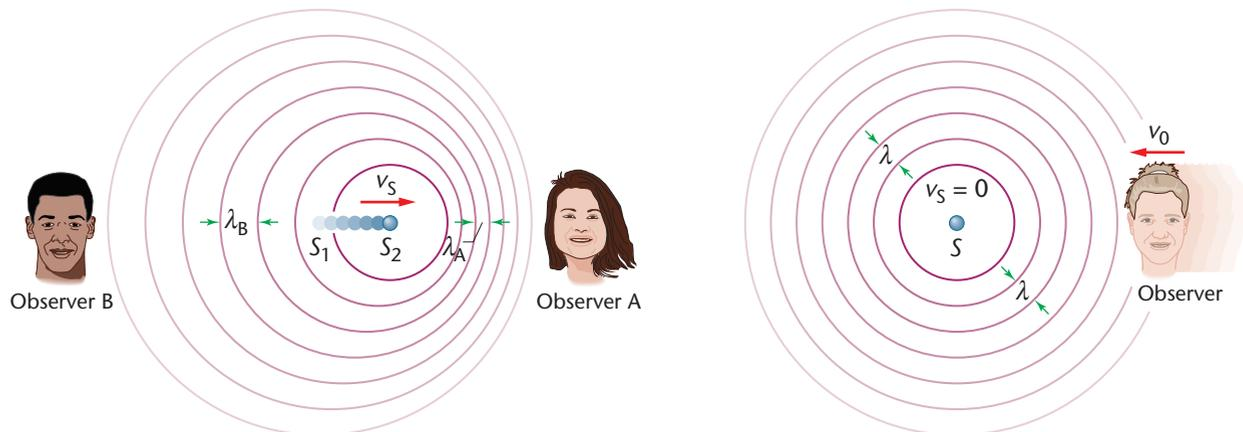
**FIGURE 15-5** A Doppler shift can be produced either by the source moving **(a)**, or by the receiver moving **(b)**.
