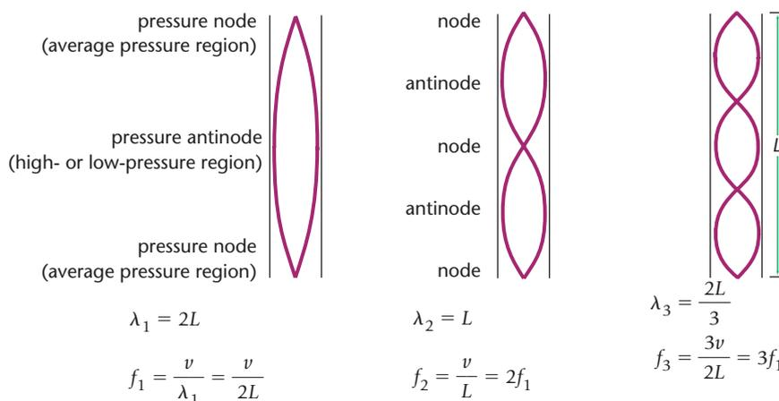
**FIGURE 15–12** An open pipe resonates when its length is an even number of quarter wavelengths.
