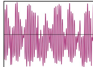
**FIGURE 15–19** Noise is composed of several frequencies and involves random changes in frequency or amplitude.
