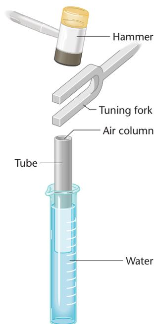
**FIGURE 15-8** Raising and lowering the tube changes the length of the air column. When the air column is in resonance with the tuning fork, the sound is loudest.
