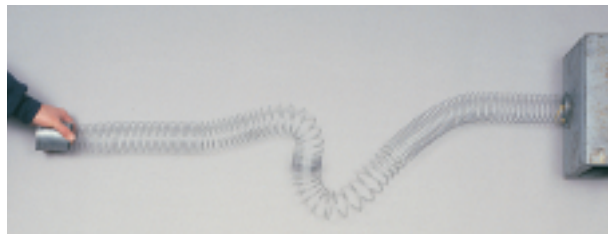
FIGURE 14–8 A pulse approaches a rigid wall (a) and is reflected back (b) . Note that the amplitude of the reflected pulse is nearly equal to the amplitude of the incident pulse, but it is inverted and appears as a downward curve.
