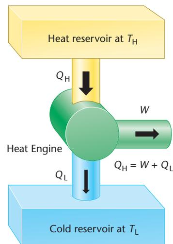
**FIGURE 12–12** This diagram represents heat at high temperature transformed into mechanical energy and low-temperature waste heat.
