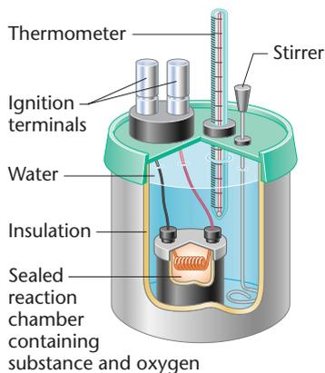
**FIGURE 12–8** A calorimeter provides a closed, isolated system in which to measure energy transfer.
