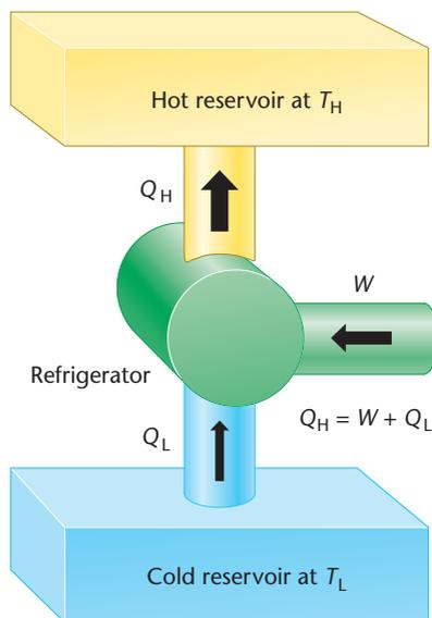
**FIGURE 12–14** A refrigerator absorbs heat  $Q_L$  from the cold reservoir and gives off heat  $Q_H$  to the hot reservoir. Work,  $W$ , is done on the refrigerator.
