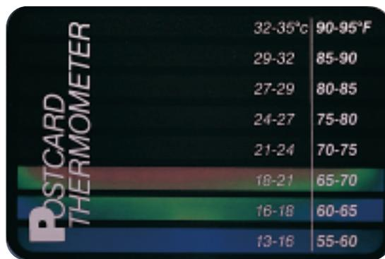
**FIGURE 12–5** Thermometers use a change in physical properties to measure temperature. A liquid crystal thermometer changes color with temperature change.
