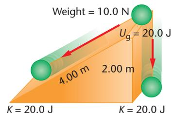
**FIGURE 11–9** The path an object follows in reaching the ground does not affect the final kinetic energy of the object.
