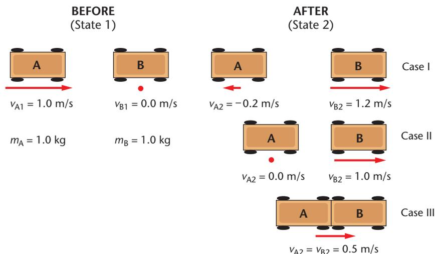
**FIGURE 11–11** The energy considerations in these three kinds of collisions between a moving object and a stationary object are different. In Case I, the two objects move apart in opposite directions. In Case II, the moving object comes to rest, and the stationary object begins to move. In Case III, the two objects stick together and move as one.
