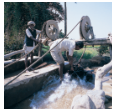
FIGURE 10–8 The pulley system makes work easier not by increasing the force the man can apply to the resistance, but by allowing him to apply the force parallel to displacement.
