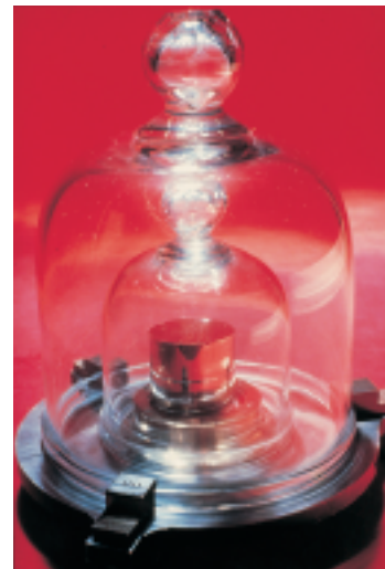
FIGURE 2-2 The International Prototype Kilogram is composed of a platinum-iridium alloy.
